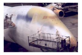
The structure of the aircraft is returned to its initial state with peraluman or avional sheets totally free of paint.
